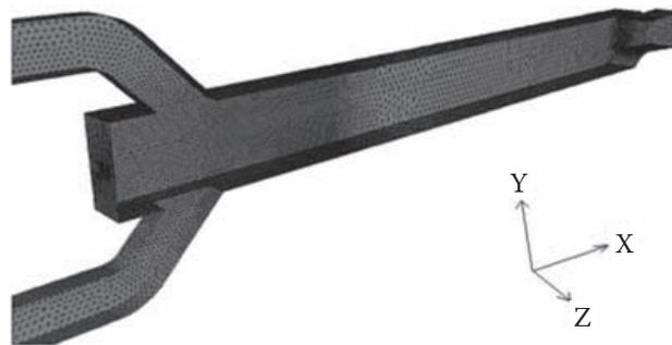
FIGURE 7.2 Three-dimensional view of the ramjet combustor mesh. (Roux et al. 2008; with permission from Elsevier Science Ltd.)
